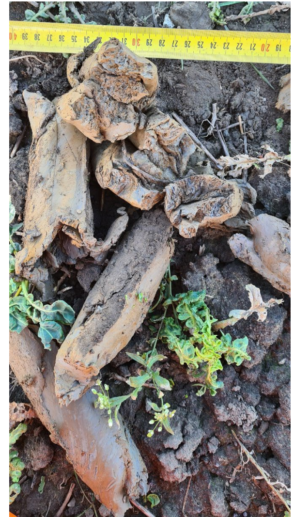
clay observed by auger
